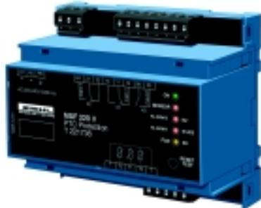
The MSF 220 V is particularly suitable for the temperature monitoring at dry transformers. 3 PTC-circuits with different nominal response temperatures (NRT) can be connected to this unit, one for controlling an fan (forced cooling) and two for alarms.
