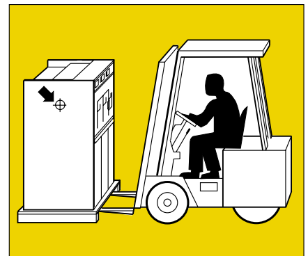
Transport of switchgear with pallet
