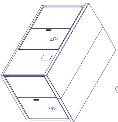
MODULE MONOBLOC EN CCV (COMPOSITE CIMENT-VERRE) AVEC CAVE A CABLES PREFABRIQUEE MUR ET TOITURE EN OREPI PORTES EN TOLES GALVANISEES PEINTES (BEIGE CLAIR)
